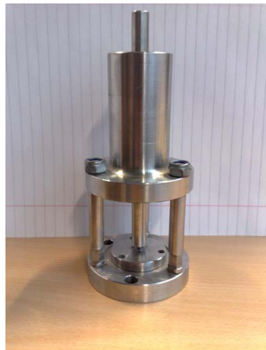
Fig. 2 Assembled ASTM F 394 test jig, no specimen installed
